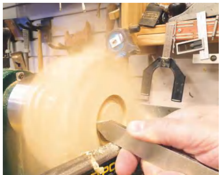
I cut the recess diameter with a parting tool before removing the waste
